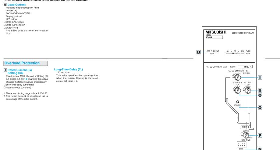
This overview lists the maximum possible functionality of the units. The following functions are included as standard equipment: 1. Displays Load current indicator 2. Protective functions Overload protection (long-time-delay) Short-circuit protection (instantaneous) 3. Peripherals Short-time-delay operation inhibit button Test terminal
