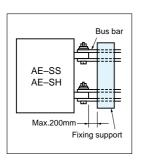
When selecting conductors for connection to a Series AE breaker, ensure that they have a sufficient current capacity, refer to Table on the right.
