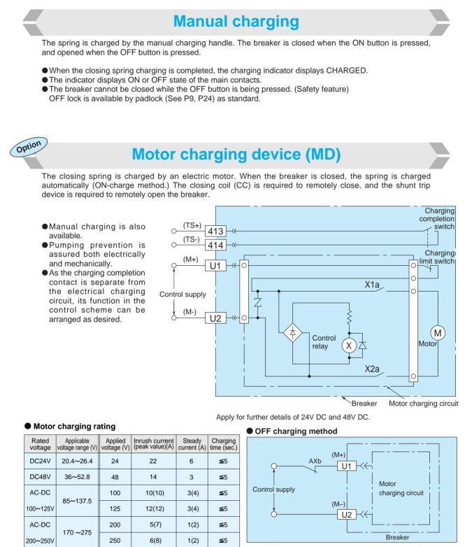
A OFF charging method is also available. The closing spring is charged automatically when the breaker is opened. This is available only by externally connecting in series b contact (AXb) of the auxiliary switch to the motor charging circuit.
