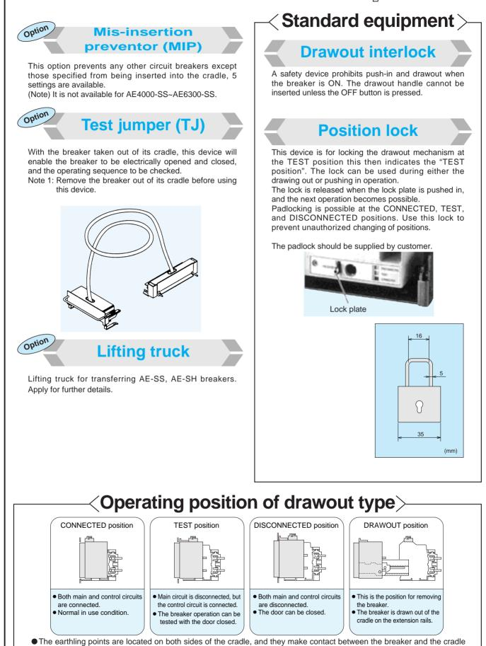
at CONNECTED, TEST, and DISCONNECTED positions.
